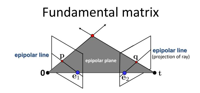
Two Special points: e<sub>1</sub> and e<sub>2</sub> (the *epipoles*): projection of one camera into the other
