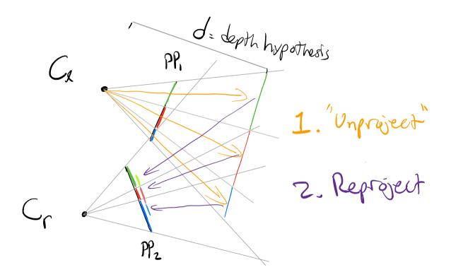
In Practice: Because the 3D object is Planar, We can move it arbitrarily with a homography. I. Find the homography a. Unproject-Then reproject the 4 corrus of Ce b. Fit a homography from the 4 correspondences.
