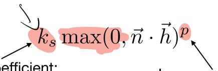
specular coefficient: determines strength of specularity term
