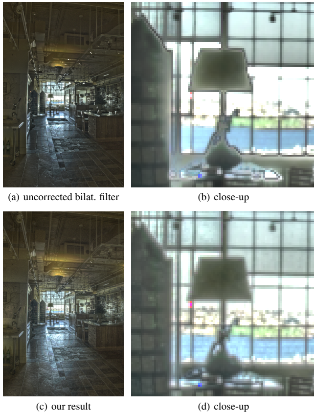
Figure 12: The bilateral filter sometimes over-sharpens edges, which can lead to artifacts (b). We used code provided by [Paris and Durand] and multiplied the detail layer by 2.5 to generate these results. Although such artifacts can be fixed in post-processing, this introduces more complexity to the system and requires new parameters. Our approach produces clean edges directly (d). We set our method to achieve approximately the same visual result ( \sigma_r = \log(2.5) , \alpha = 0.5 , \beta = 0 ).
